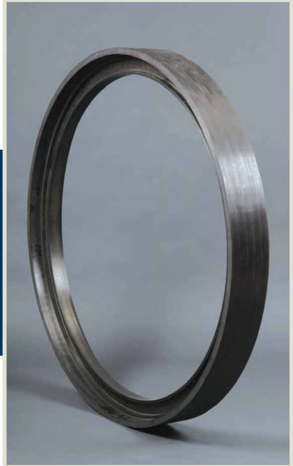
▲ Composite I-Beam Stiffened Cylinder Section
